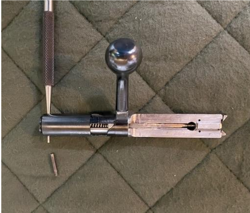
Figure 13 Compressed spring captured with a punch
