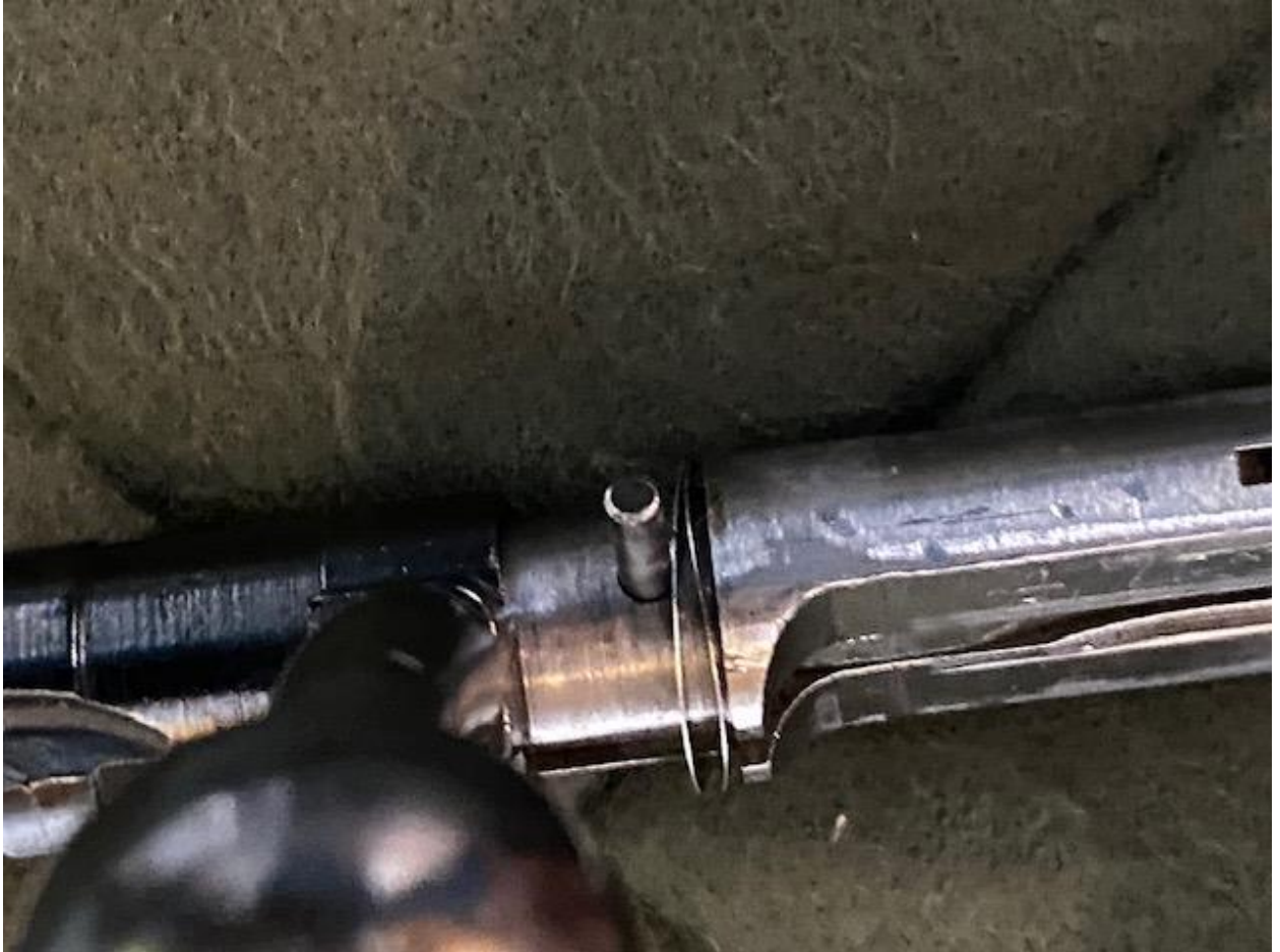
Figure 11 Installation of the firing pin stop pin
