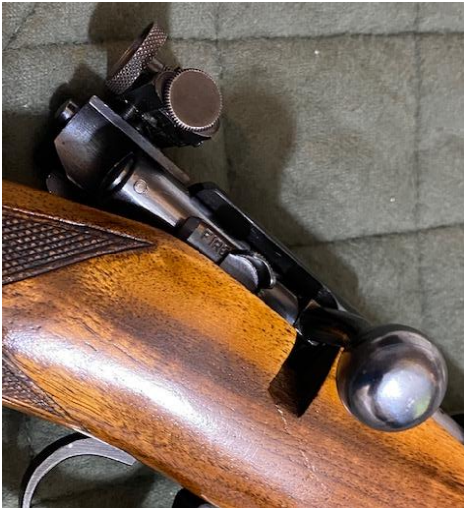
Figure 19 Bolt NOT Able to Close with NO GO Gauge
