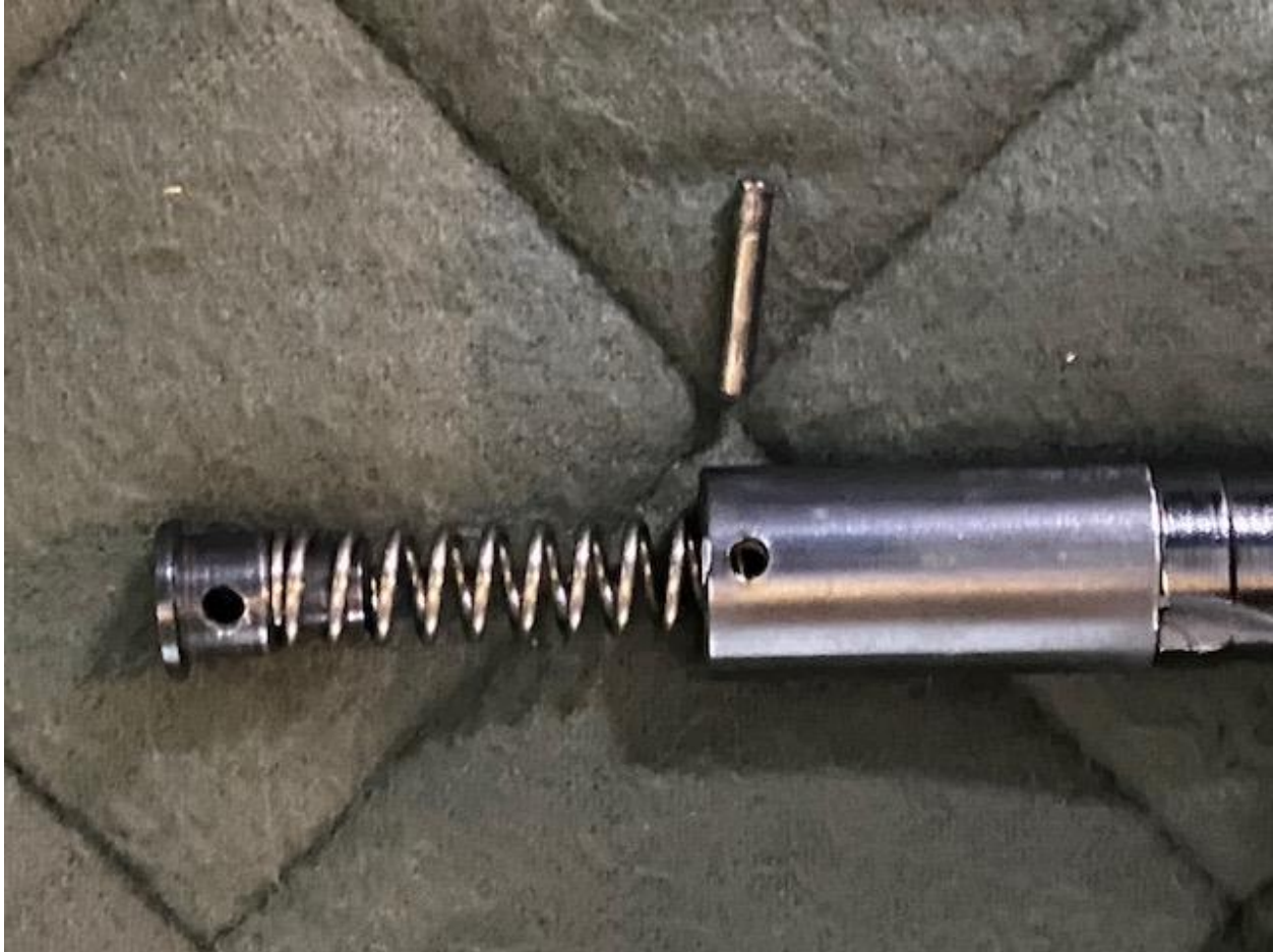
Figure 12 Preparation for Breech Bolt Sleeve Pin installation
