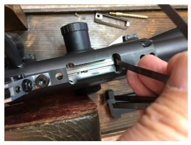
I could probably stop here. I'm sure you have this figured out. Just add the two measurements you have just taken together and that is the headspace for this specific rifle. In the case of my CZ 457 a .009" feeler gauge was a very snug fit. So the .037" recess in my bolts face and the .009" distance between the bolt and barrel sum to a headspace of .046".
