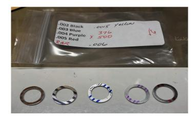
I disassembled my bolt and slipped the thickest of the five shims (.005") over the firing pin and then into place on the bolt (I'd measured the gap at .004" but decided to try the thicker shim "just in case").
