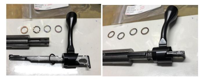
As expected, after I reassembled the bolt I found I couldn't open the bolt handle all the way because the .005" shim was too thick:
